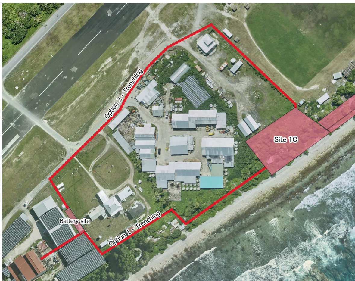
Figure 9: Options 1 & 2 routes for trenching the cable from the solar PV panel to BESS and grid system.
